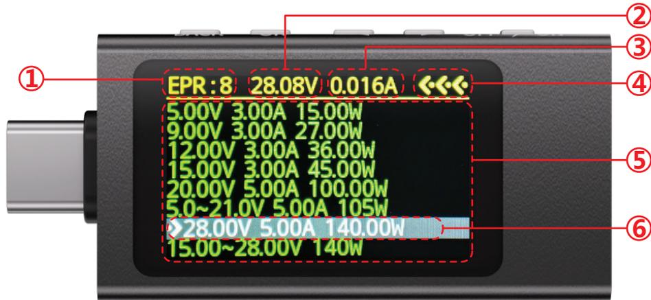
Note: The gear selected here with (+/-) will not trigger immediately; it requires pressing the (Confirm) button again to confirm the deception, which will then be displayed at the top and the operation executed. Display color (red + green) follows the above logic.
