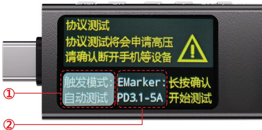
1. Trigger the default tab, (+/-) to switch, (Confirm) to select.
