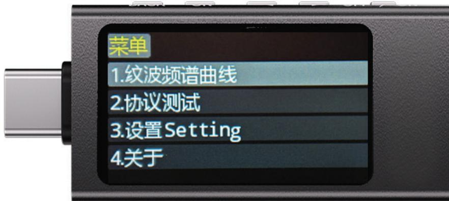
Entry condition: In the "Home - Measurement" screen, long press the (Back) button.
