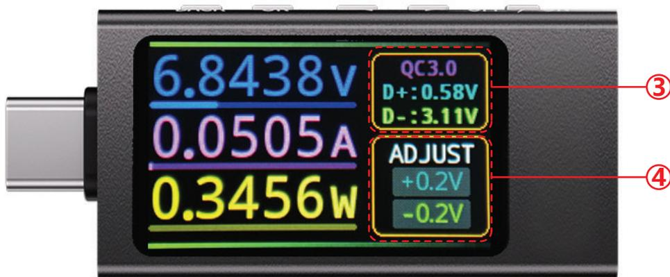
Note: QC2.0 has fixed gears, while QC3.0 and QC4+ support 200mV step adjustment, corresponding to 0.2V as the minimum adjustment unit.
