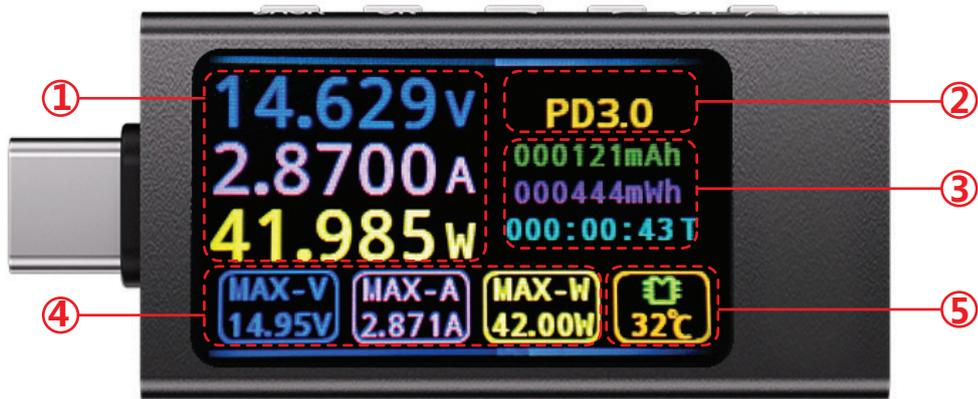
1. Real-time display of voltage, current, and power.
